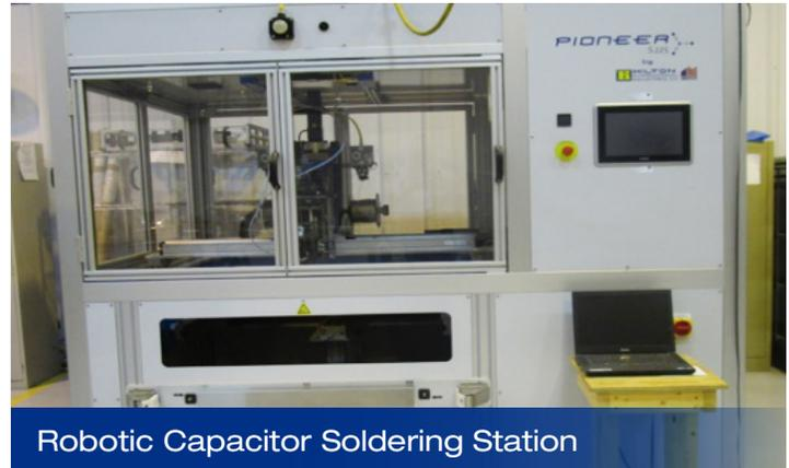
Robotic Capacitor Soldering Station
